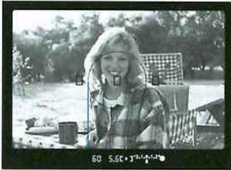
Partial metering circle
